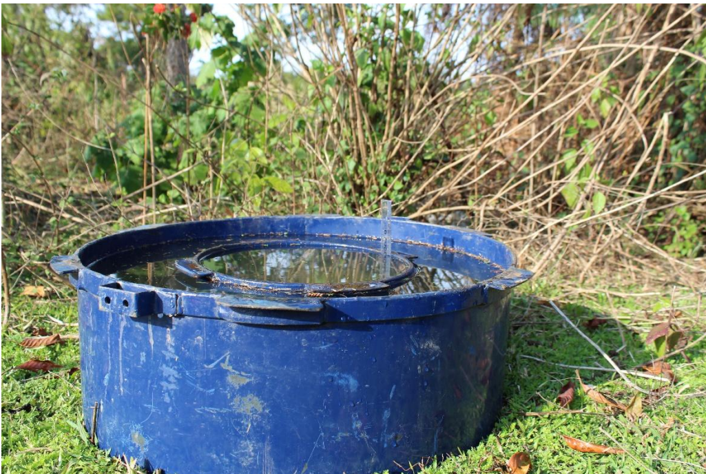
Soil Infiltration Test Studies in West Jaintia Hills
